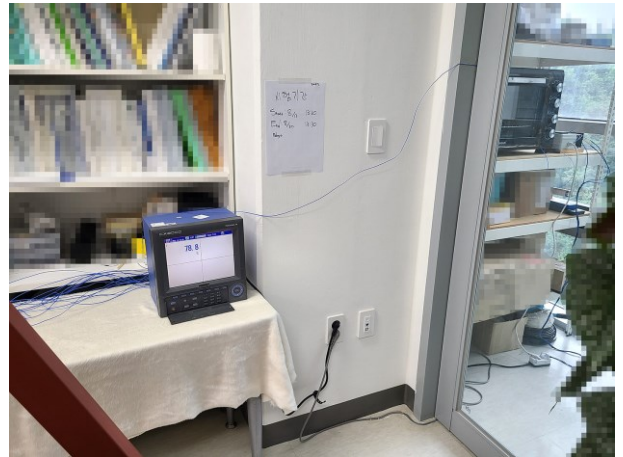
<Temperature measurement during 17 days at 80°C>
