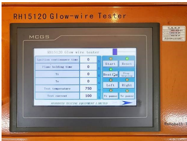
<Glow-wire test: 750 °C setting>
