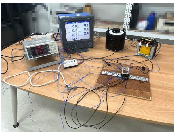
<Temperature rise test>
