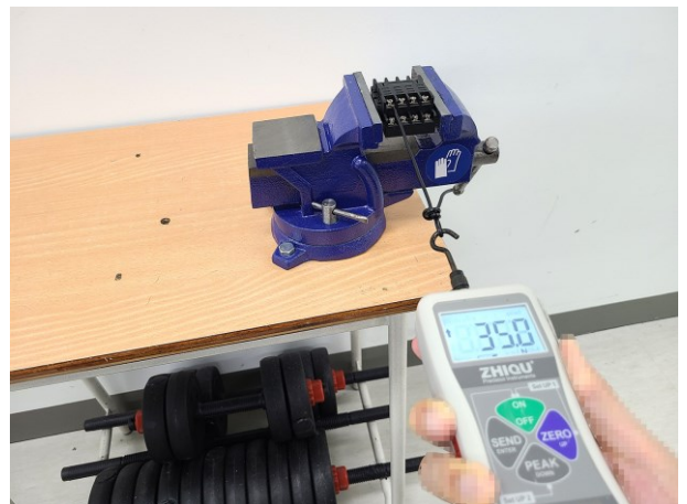
<Pulling out for 1 minute at 35 N>
