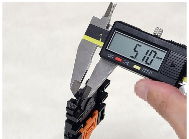
<Insulation distance: KH-RS-H4C>
