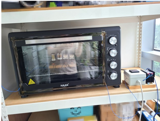
<7 days of ULT + 240 h of IEC 61810-1 requirement at 80 °C>
