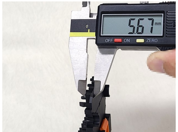
< Insulation distance: KH-RS-H4CS>
