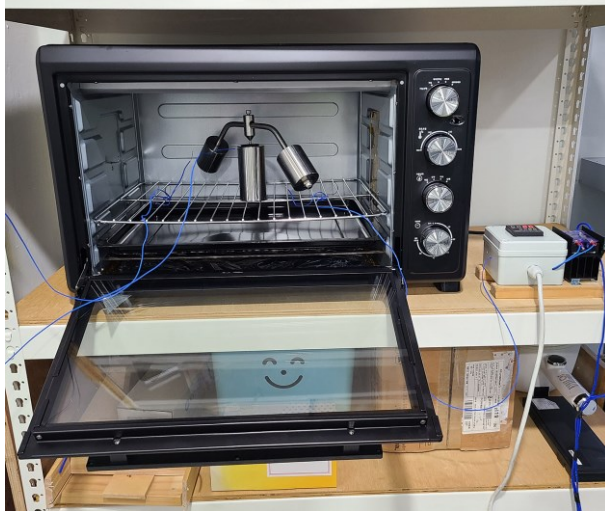
<Ball-pressure test setup>
