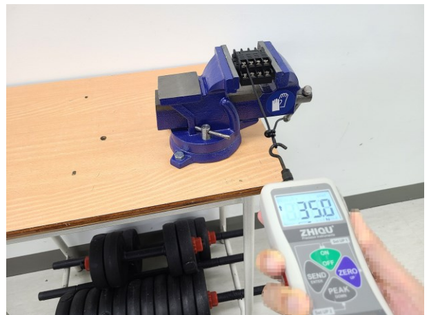
<Pulling out for 1 minute at 35 N>
