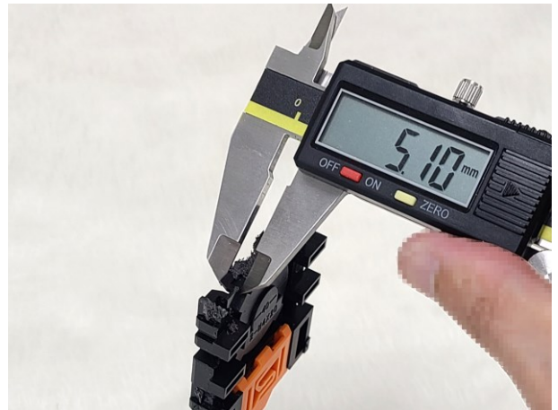
<Insulation distance: KH-RS-H4C>
