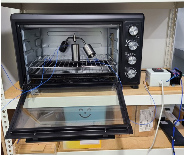
<Ball-pressure test setup>
