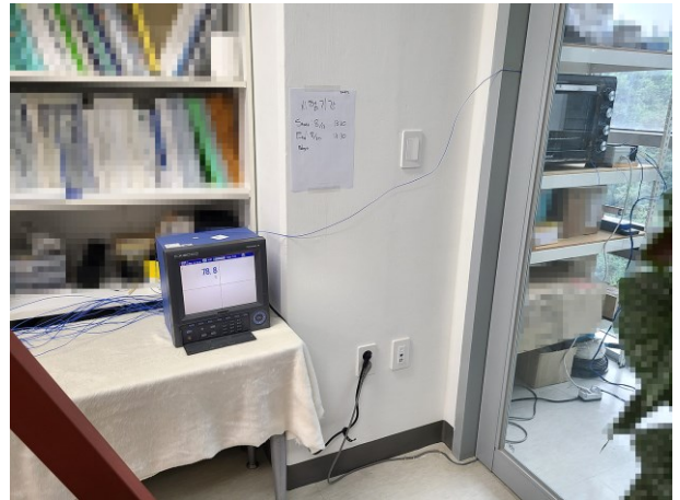
<Temperature measurement during 17 days at 80°C>
