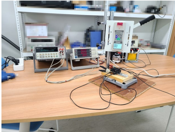
<Mechanical operation & contact resistance setting>
