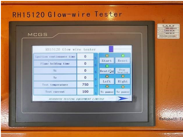
<Glow-wire test: 750 °C setting>
