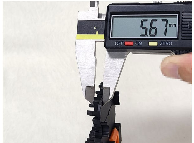
< Insulation distance: KH-RS-H4CS>
